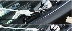
8. To remove the inner door handle cable pull out on the 2 plastic tails and push the clip left
