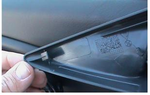
**6.** With the bolts, screws and mirror panel removed the door panel can be removed by popping the plastic clips on the outer edges of the panel and sliding it up off of the window frame.
