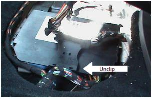
5. To release the module remove the plastic phillips head screw on the left side of the module
